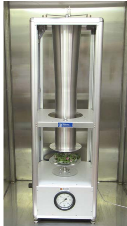
Figure 1. The Potter precision laboratory spray tower used in pesticide applications.
